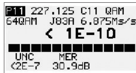
Digital measurements : BER MER in QAM
