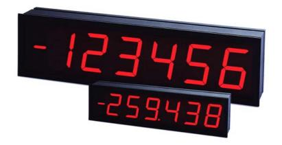
Displays OC57-DC, Large OC100-DC and OC125-DC are 4- or 6-digit programmable instruments with up to ±200000 measuring increments. They have inputs for DC signals, strain gauges, 4-20mA loops, ±100mV etc. and are available with 57mm, 100mm or 125mm large 7 segment display units. Due to the free scaling, the input signals can be displayed in units corresponding to the measured process, such as kg, gr, lb, kN, MPa etc.
