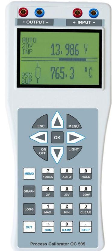
**OC505** is a Calibrator-Multimeter for generation of Currents 0-22mA Sink or Source and Voltages to 25VDC. External voltages  $\pm 2V$ ,  $\pm 20V$  and  $\pm 200VDC$  (firm ranges or auto ranging) and Currents to 0-100mA can be measured simultaneously and shown at the display.
