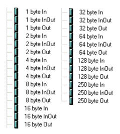
Adjust the necessary "total I/O data width" with any combination of the modules above (max. 4). Therefore "drag" the I/O-modules into the slots of the Profinet interface and obey that a maximum of 250 output- and 250 input-bytes are allowed.
