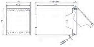
Installation Fastening Snap-on fastening on top hat rail 35 mm accord. to DIN EN 60715
